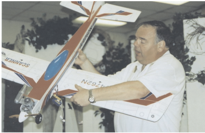
Bob Wade, W6RTW holds up one of his gas powered model planes displaying the mini sized 6 meter receiver used to control the plane.
