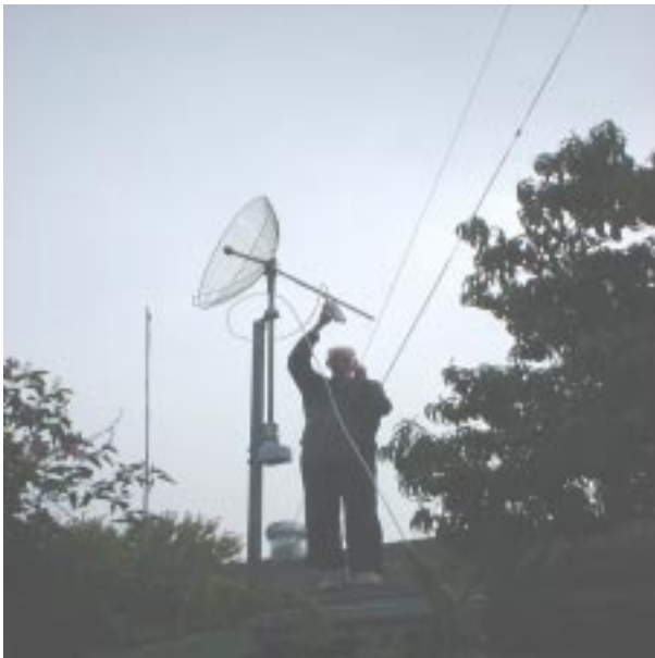
K6LG holding 2.4 GHz downconverter and antenna elevation adjustment string.
