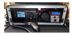
A Bioenno 30Ah LFP Battery (*PVC*, *BLF-1230A*) is strapped to the frame and an *Epic-H PWRgate* is used to maintain the battery. There is a Bioenno 28 watt foldable solar panel (*BSP-28*) stored on top of the rig that provides 15-18 volts at 1.55A. Two BSP-28 panels can be chained together to increase the output maximum current to 4A.
